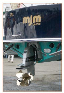
**Safety** The Standard 29z includes sturdy stainless bowrails. A solid swim platform suppresses exhaust and prop noise as well as being an important safety feature. If one falls overboard with nobody near to help, a custom Armstrong telescoping swim ladder with transom handle makes reboarding easy. A benefit of a sterndrive that can be raised is: one can clear pot warps or a fouled prop by kneeling on the platform rather than having to go swimming in cold water.
