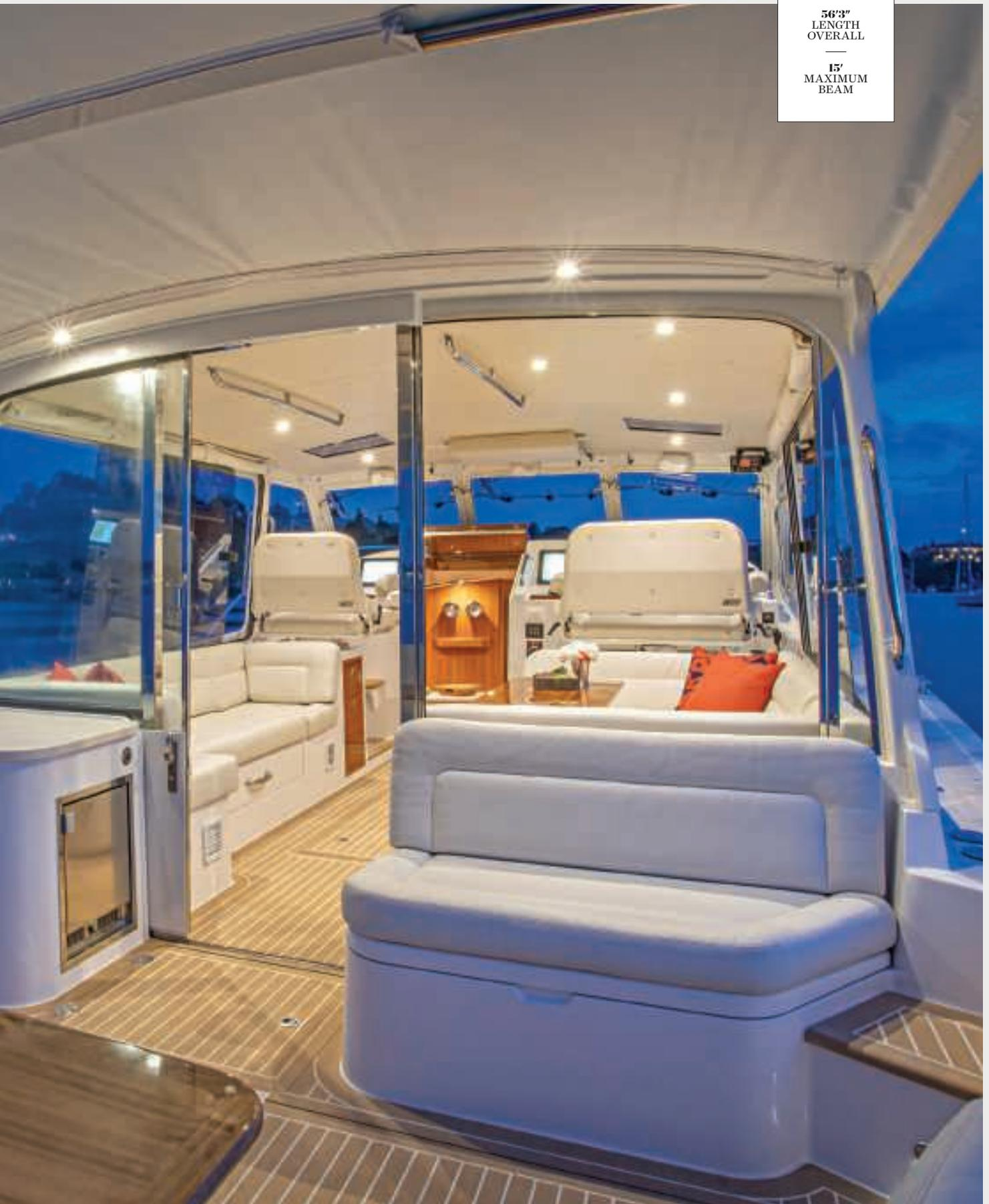
The steps from the cockpit to the side decks are 11 inches in height. The salon's 30-inch-wide pocket door saves valuable cockpit real estate.
