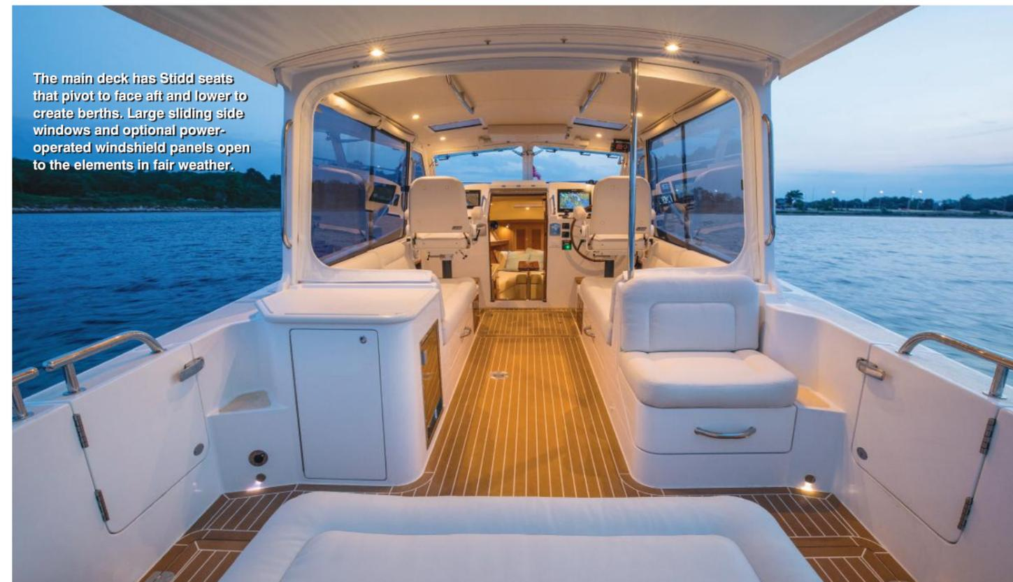
The main deck has Stidd seats that pivot to face aft and lower to create berths. Large sliding side windows and optional power-operated windshield panels open to the elements in fair weather.
