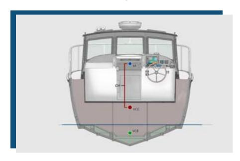
The most influential factor in a vessel's initial (static) stability is Metacentric Height (GM). This is the distance between Metacenter (M), the location of which is fixed by a vessel's form stability and Vertical Center of Gravity (VCG). VCG is determined by the vessel's shape and quality of construction. The lower the VCG, the more stable the vessel. That's the key to MJMs. By using stronger, lighter epoxy composite laminates, and
