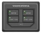
START ENGINES by pushing the START/STOP button. Note: If you can't hear the engines (These are quiet boats), look at the RPM on the display to see that it climbs to 600-700. The engine will not start unless the shift levers are in NEUTRAL.
