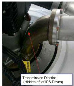
**ACAUTION** Be sure not to overfill this reservoir as damage to the engine could result.
