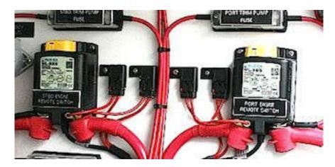
Starting with all ignition and battery switches OFF again. Turn the House Battery and Engine Battery switches ON (not the EEP switch). Then go into the central pilothouse hatch and push the yellow button on top of the PER switch down until it clicks in place. Proceed with turning the Engine Ignition switches ON. Check for equal, good voltage on the Engine Displays. START the engines.
