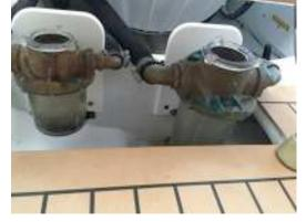
should be checked with frequency...particularly in weedy areas daily. These strainers keep seaweed and other particles from plugging up engine cooling systems and causing overheating and potentially severe damage.
