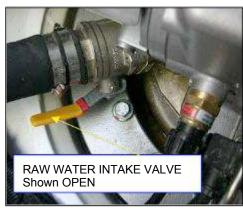
zinc periodically at the time of oil changes and remove the corroded area on the surface, replacing them when deteriorated to less than 50% of original size. Otherwise corrosion-cooling system will occur and water leakage or parts breakage will result. Be sure to close the raw water intakes at the base of drives, before removing a plug to replace a zinc.
