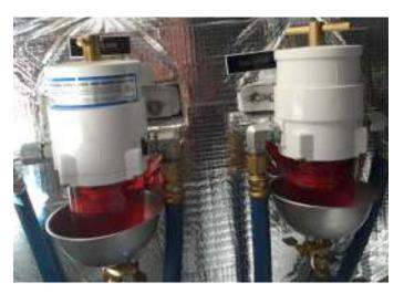
FILTER ACCESS LID – Be sure to close fuel shut-off valve before opening. Be careful to seal properly without pinching gasket.
