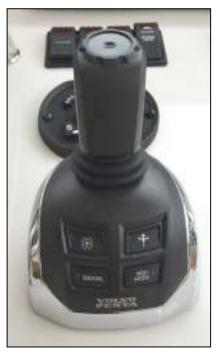
**Boost Function** In windy weather or current when you need more oomph, push the lower right "HIGH MODE" button after having first activated the "Docking" button. A beep will confirm it's engaged. Deactivate by pushing the button again. You'll hear a double-beep confirmation.
