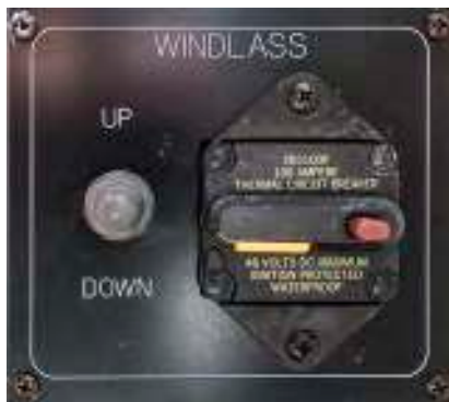
WINDLASS control panel at helm
