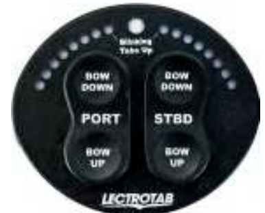
TRIM TAB CONTROL panel
