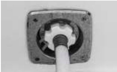
DOCKSIDE HOSE INLET with a hose connected
