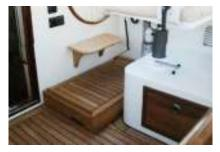
**Esthec Riser (Option)** This 4" high removable riser improves visibility for someone shorter than 5'5". It locks into place with a barrel bolt and can be stored in one of the settee lockers.
