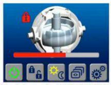
To start, press the POWER ON/OFF. A RED PROGRESS BAR will appear. When the GYRO reaches operating speed the PROGRESS BAR will turn. GREEN, The GYRO is available for stabilization.
