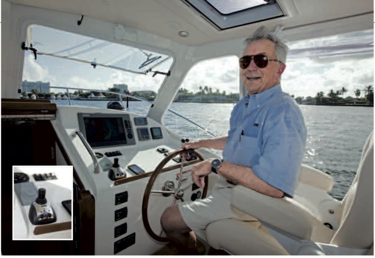
Above: Bob Johnstone at the wheel of the MJM 36z. The all-important IPS joystick (inset) is set amidships for easy use when facing aft and backing into a slip. Right: With both forward windshields open, the pilothouse turns into what Johnstone calls 'a flying bridge without a ladder.'
