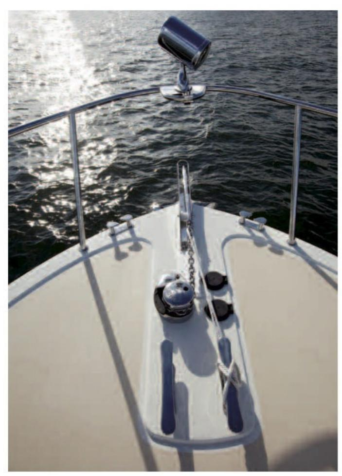
Above: A low-profile Muir anchor windlass, with an auto-launching plow anchor and washer system, is set amidst oversized cleats and chocks. Right: The sturdy stainless steel bow rail is topped by an optional remotecontrol spotlight.
